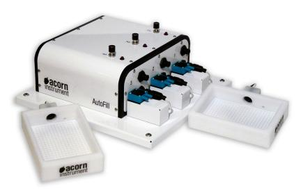
**AutoFill Reservoirs** are reagent troughs that keep themselves filled. Each reservoir has an embedded sensor which monitors its liquid level. When needed, a controller refills the reservoir by adding reagent via a miniature pump. If source reagents run out and the reservoirs cannot refill, no problem, the controller can be configured to send emails or raise events enabling your automation software to notify you and pause a run.
